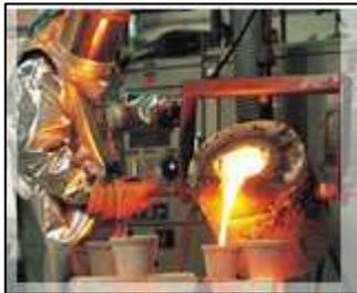
1. Vacuum induction melting of elemental constituents (Ni, Ti, Pd, Sc)
