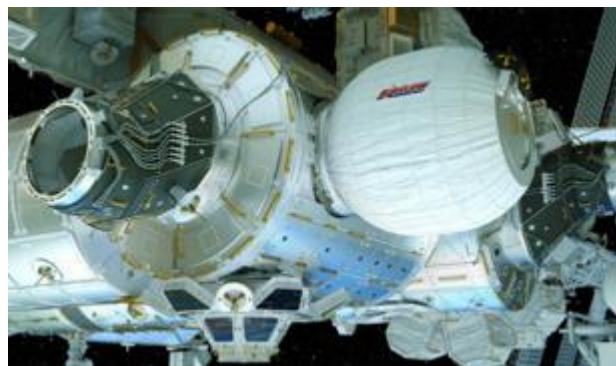
Fig. 2: The BEAM module will be attached to the rear port of the space station's Node 3. After installation, the BEAM expands to roughly 13-foot-long and 10.5 feet in diameter. Credits: Bigelow Aerospace, LLC
